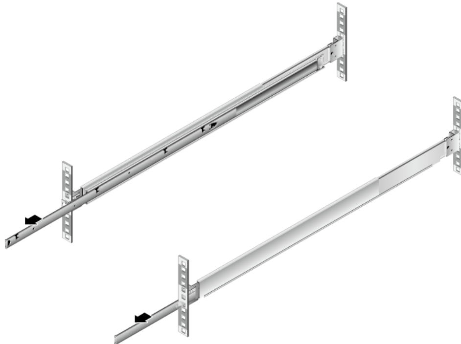
Figure 7-9 Pulling out inner rails
